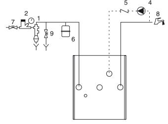
Connection without thermostatic mixing valve
