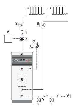
Hydraulic diagram with circulator controlled by a room thermostat.
