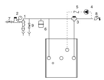
Connection with thermostatic mixing valve
