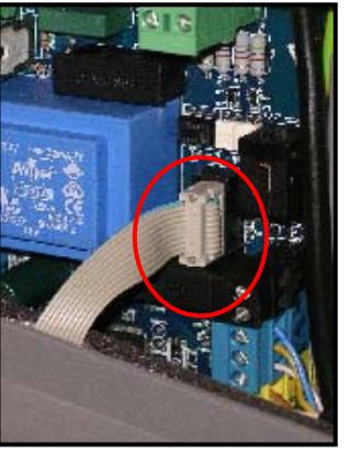
Remove the display connector from the PCB.
