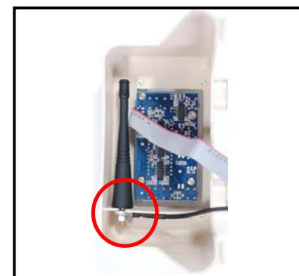
Fit the aerial cable to the side of the RF aerial between the two washers!!!! Then fit the serrated lock washer to the aerial.
